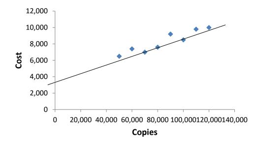
The line intersects the y-axis at \$3,500, representing total fixed costs. The line passes through the point (80,000, \$7,600), so the slope can be calculated as follows:
