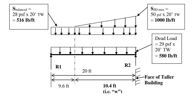
Using principles from statics, we can calculate the girder reactions as follows:
