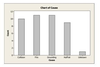
Fire and grounding are the two most likely causes of puncture.
