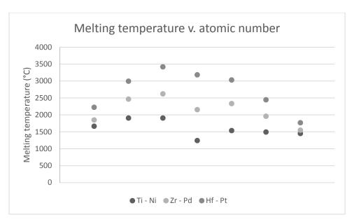
For each row, the melting temperature is highest when the outer "d" energy level is partly full. In Cr, there are 5 electrons in the 3d shell; in Mo, there are 5 electrons in the 4d shell; in W there are 4 electrons in the 5d shell. In each column, the melting temperature increases as the atomic number increases—the atom cores contain a larger number of tightly held electrons, making the metals more stable.
