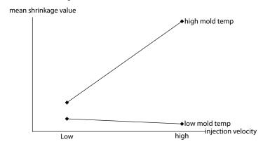
It is quite obvious to find the interaction between the two variables. Since in this experimental data, those two variables can be controlled each at two levels, the interaction can be inves-
