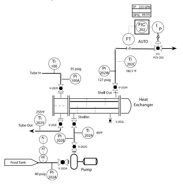
15. Draw a simple sketch of a shell and tube exchanger. Show all flows: tube-in, tube-out, shell in, shell out, shell, channel-head, pass partition, tube-sheet, and all associated valves. Explain principles of heat transfer, flow rate, and pressure and illustrate on your drawing how they work.
