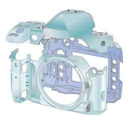
This was most likely manufactured using a die cast procedure because of the material and geometric detail in the pieces including a number of inclusions. Certain features could have been machined, and some polishing/grinding operations may have been used.
