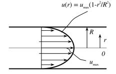
Note that the quantity du/dr is negative in pipe flow, and the negative sign is added to the  $\tau_w$  relation for pipes to make shear stress in the positive (flow) direction a positive quantity. (Or, du/dr = -du/dy since y = R - r). Then the friction drag force exerted by the fluid on the inner surface of the pipe becomes
