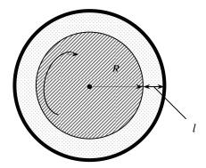
**Analysis** (a) The radius of the shaft is R = 0.05 m, and thickness of the oil layer is  $\ell = (10.3 - 10)/2 = 0.15$  cm. The power-torque relationship is
