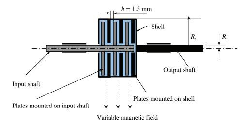
**Analysis** (a) The velocity gradient anywhere in the oil of film thickness h is V/h where  $V = \omega r$  is the tangential velocity relative to plates mounted on the shell. Then the wall shear stress anywhere on the surface of a plate mounted on the input shaft at a distance r from the axis of rotation is expressed as
