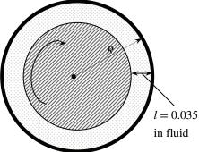
**Assumptions** 1 The inner cylinder is completely submerged in the fluid. 2 The viscous effects on the two ends of the inner cylinder are negligible. 3 The fluid is Newtonian.
