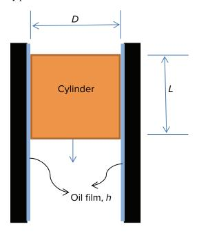
Analysis Assuming a linear velocity profile in the oil film the drag force due to wall shear stress can be expressed as
