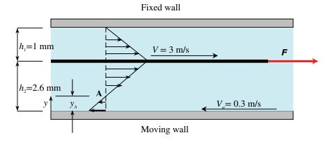
(b) The magnitudes of shear forces acting on the upper and lower surfaces of the plate are
