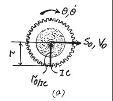
Also, from Fig.  $a, v_O = \dot{\theta} r_{O/IC} = \dot{\theta} r$ . The mass moment of inertia of the gear about its mass center is  $I_O = mk_O^2$ .
