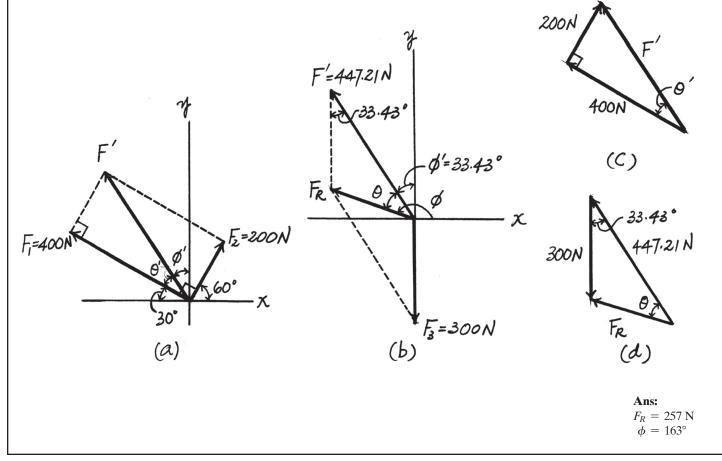
\*2–20. Determine the magnitude and direction of the resultant force,  $\mathbf{F}_R$  measured counterclockwise from the positive *x* axis. Solve the problem by first finding the resultant  $\mathbf{F}' = \mathbf{F}_2 + \mathbf{F}_3$  and then forming  $\mathbf{F}_R = \mathbf{F}' + \mathbf{F}_1$ .
