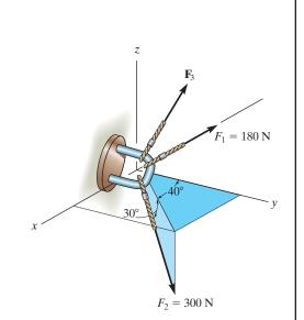
**2–69.** Determine the magnitude and coordinate direction angles of  $\mathbf{F}_3$  so that the resultant of the three forces is zero.
