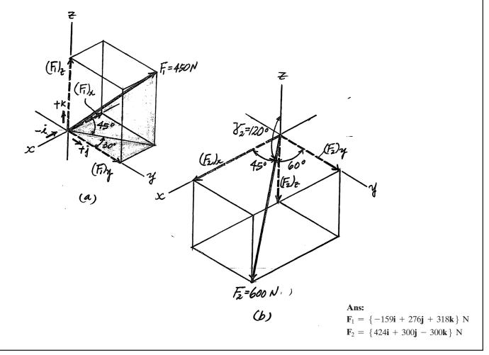
**2–61.** Determine the magnitude and coordinate direction angles of the resultant force acting on the bracket.
