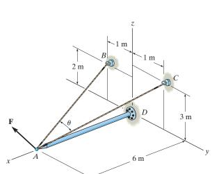
\*2-120. Determine the magnitude of the projected component of force  $\mathbf{F}_{AB}$  acting along the *z* axis.
