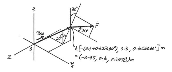
**2-138.** Cable *OA* is used to support column *OB*. Determine the angle  $\theta$  it makes with beam *OC*.
