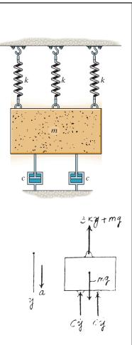
Ans:  $\ddot{y} + 16\dot{y} + 12y = 0$ Since  $c > c_c$ , the system will not vibrate. Therefore it is **overdamped**.
