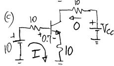
$J_{C=0} \Rightarrow J_{B=JE} = I$ . kVL:  $10=10I + 0.7 + 10I \Rightarrow I = 0.465 mA$   $\Rightarrow V_{E} = 4.65V$ ,  $V_{B} = 5.35V$ .  $\forall 0 \downarrow c = 0$ ,  $V_{CC} = V_{B} - 0.65 = 4.7V$ .
