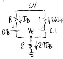
VE=2×2778=54 B. R\$\f\text{IB} \langle \frac{1}{5} \delta \frac{1}{26} \text{IB} \rangle \frac{1}{5} = \frac{1}{26} \text{IB} + 0.1 + 54 \text{IB} \Rightarrow \text{I}\_B = \frac{61.25}{18} = \frac{61.25}{18} \text{A.}
