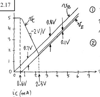
① FOR  $V_{\pm} < V_{BE(EOC)} = 0.6V_{j}$ the BJT is in cutoff;  $V_{C} = V_{S} = 5V_{j}$ , ic = 0.
