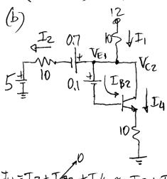
$\frac{12 - Vx}{10} = \frac{(Vx - 0.7) - 5}{10} + \frac{(Vx - 0.1) - 0.7}{10} \Rightarrow Vx = 6.16 V.$  $IB_1 = I_2 = \frac{(6.16 - 0.7) - 5}{10} = 0.046 \text{ mA}; I_{C2} = I_4 = \frac{(6.16 - 0.1) - 0.7}{10}$ =0.536 mA. Ic1=IBZ= Tc2/BF2. Assuming BF2>100, Me have Ic1 < 0.536/100 = 5.36μA >β sol1 < 5.36/46.6 ~0.1 => Q1 = Sat. Thus, Q1=Q1 (<5.36MA, 0.1V), and Qz=Qz(0.536mA, 0.8V).
