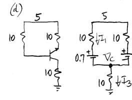
BJT is in reverse-mode Saturation. Equivalent Circuit is similar to (b).  $V_C = 3.1V$ ,  $I_1 = 0.12 \text{ mA}$  $I_2 = 0.19 \text{ mA}$ ,  $\beta_{sot} = 0.19/0.12 = 1.6$ . 2.25 [V, mA, kn].
