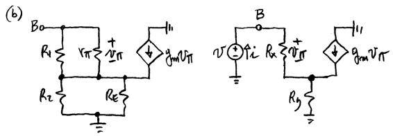
With the switch closed, we get the circuit at the left. This, in turn, is equivalent to that at the right, provided we let  $R_X = R_1 //V_T$  and  $R_y = R_2 //R_E$ . Applying a test voltage, as shown, we get, by KCL & KVL,  $\frac{V_T}{R_X} + 9mV_T = \frac{N^2 - V_T}{R_Y}$ . But,  $V_T = R_X i$ . Eliminating  $V_T$ , collecting, and taking the ratio  $R_i = \frac{T}{i}$  gives  $R_i = R_X + (1 + 9mR_X)R_Y$ .
