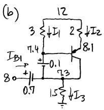
Assume  $Q_1 = Sat$ ,  $Q_2 = TA_1$ , and check.  $Ve_1 = Vc_2 = 8 - 0.7 = 7.3V$ ;  $T_3 = 7.3/1.5 = 4.87$  MA;  $Vc_1 = VBz = 7.3 + 0.1 = 7.4V$ ;  $Ve_2 = VBz + 0.7 = 8.1 \text{ V. } I_1 = (17 - 7.4)/3 = 1.53$  MA;  $I_2 = (17 - 8.1)/2 = 1.95$  MA.  $Q_2 = Q_2(1.95$  MA) 0.8V), FA. KCLi
